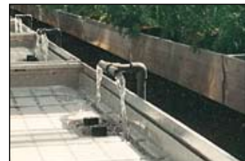
On the picture GVI's supply unit in PVC pipe is shown together with 2 siphon valves mounted on the same container table.
